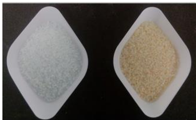
Figure 6: TiO 2 coated glass beads before (left) and after (right) photodecomposition reaction of acetone. Yellowish discoloration is due to accumulated carbonaceous species on TiO 2 surface.
